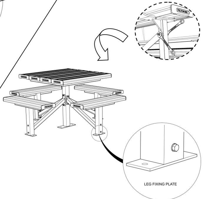
Tight all the bolts with spanner and/or proper tools as necessary.
