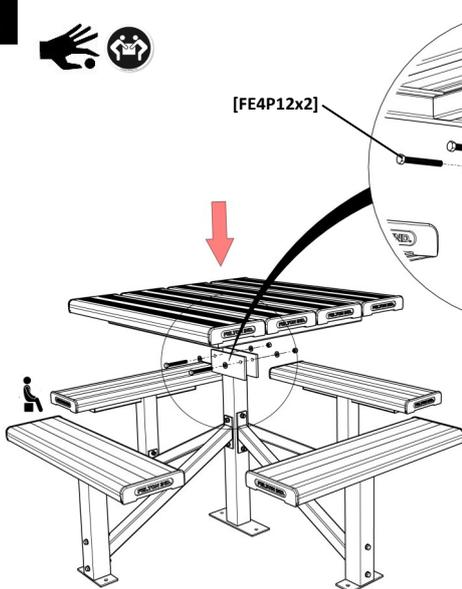
Connect the table bench assembly to the rest of the 4 pedestal park setting, as illustrated. Secure the table frame [FE4P5] to central post fixing plates, by using hexagonal head bolts [FE4P12], locknuts [FE4P15] and washers [FE4P17]- Finger tighten.
