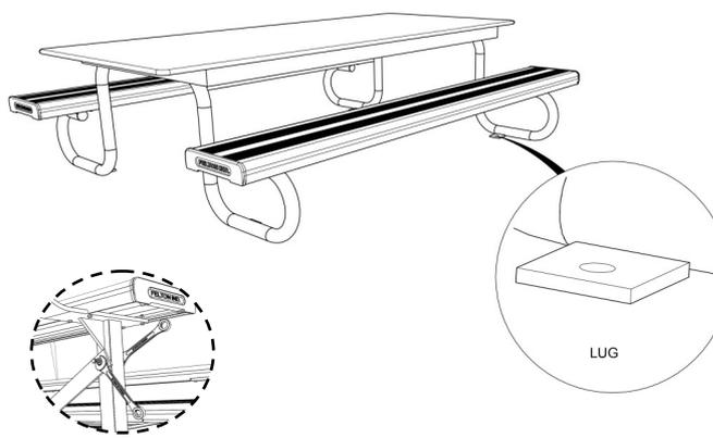
Tighten all bolting accessories with spanners and appropriate tools. Attach the whole unit to the ground, by using dyna-bolts on each frame lug.
