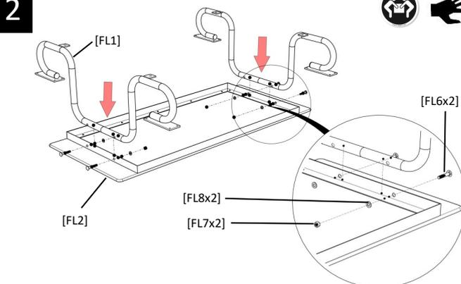
Have the main frames (FL1) frame in place, tags facing inward and connect them to the table bench (FL2), by using cup head bolts (FL6), locknuts (FL7) and washers (FL8).
