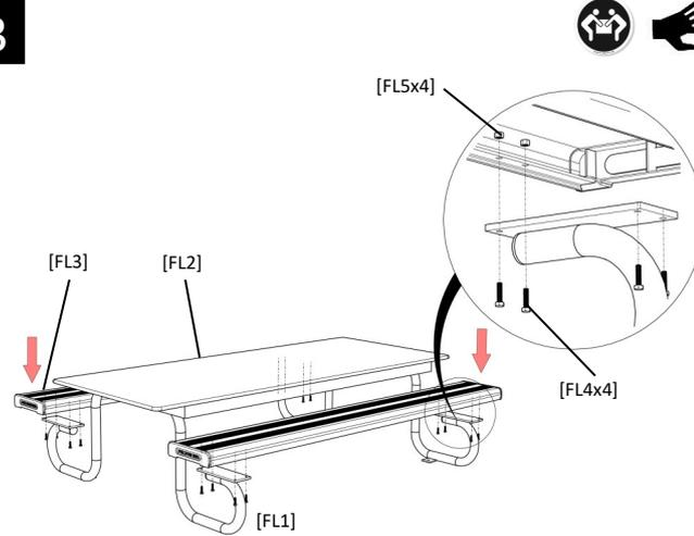
Turn the entire assembly up and connect the two seating planks (FL3) to the main legs (FL1) as shown, by using with hexagonal head bolts (FL4) and nuts (FL5).
